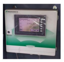
Contact-less Brasten Density analyzers are the perfect alternative of the Nuclear gauge to avoid Government regulations required for handeling a nuclear isotope and reduce the high users cost of this technology. Further with the Brasten technology you avoid a lot of difficulties to use non-contact-less sensors as Corriolis meters with possible damages dues to complex flow paths (bypass) which may lead to either blockages and erosion.
