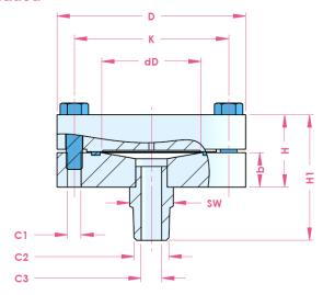
ASME 1.20.1 – NPT tapered thread
